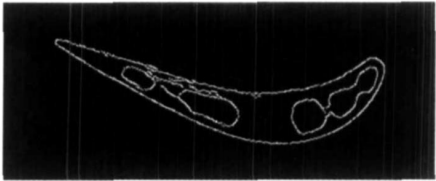
图 7 DGAUSS 算子提取的叶片边缘 Fig. 7 Edge of blade detected by DGAUSS
